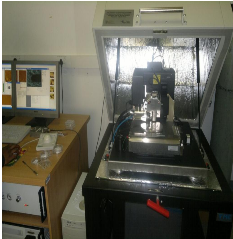
Figure 3.4: Atomic force microscopy (AFM) (Surface imaging systems, Veeco, Germany) used for determining the influence of deposited pure Zr on the surfaces of on \beta -Ti III/TIM orthodontic archwires
