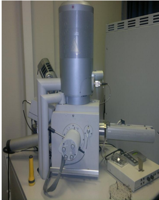
Figure 3.5: Scanning electronic microscopy (SEM) (A FEI Nova Nano SEM 230, Eindhoven, Netherlands) used for determining elemental composition of uncoated and coated \beta -Ti III/TiM orthodontic archwires with 5, 10, 25 and 50nm thicknesses of pure Zr
