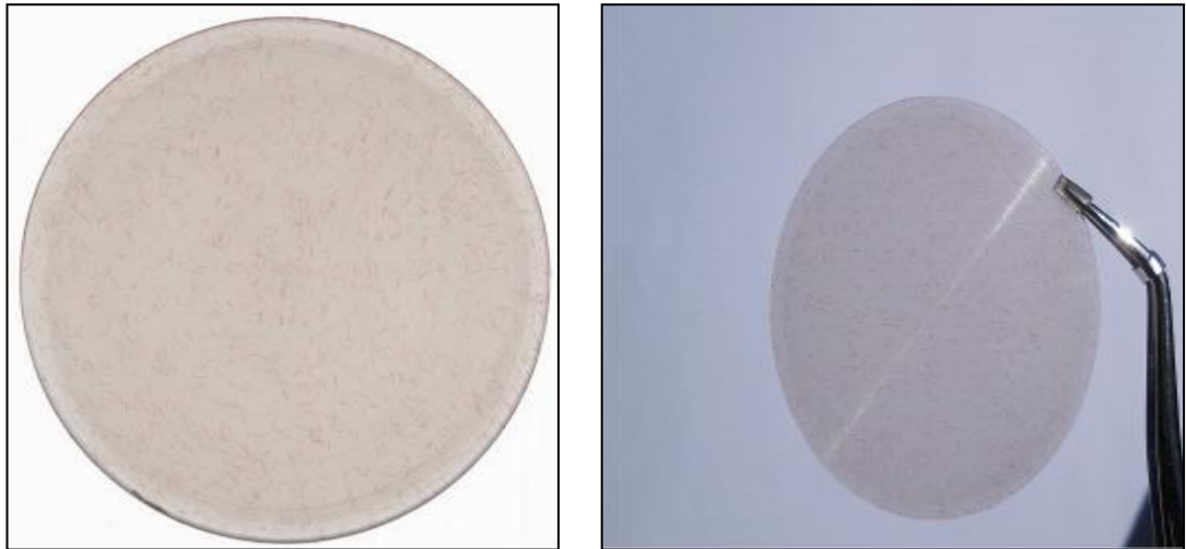
Figure 2.4: Specimen according to ISO before testing (specimen was scanned using an Epson 1680 Flatbed scanner at 1600dpi)
