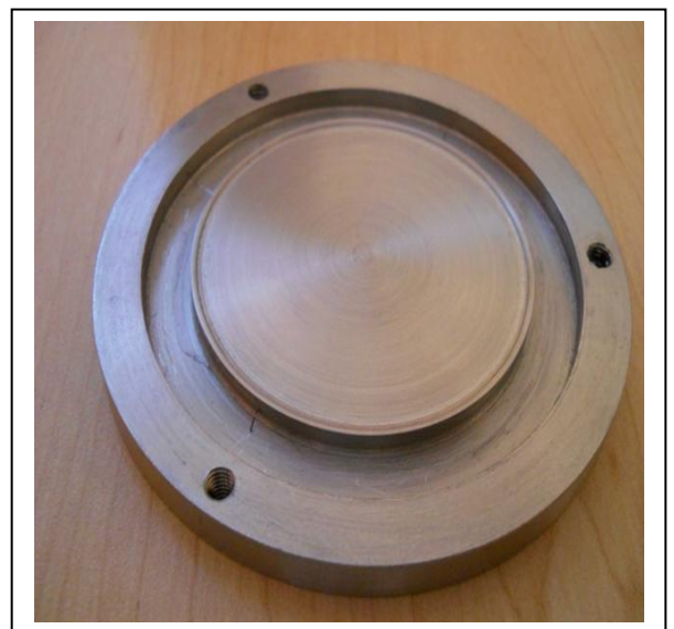
Figure 2.3: Close-up view of stainless steel mould
