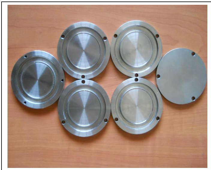
Figure 2.2: Stainless steel moulds and cover
