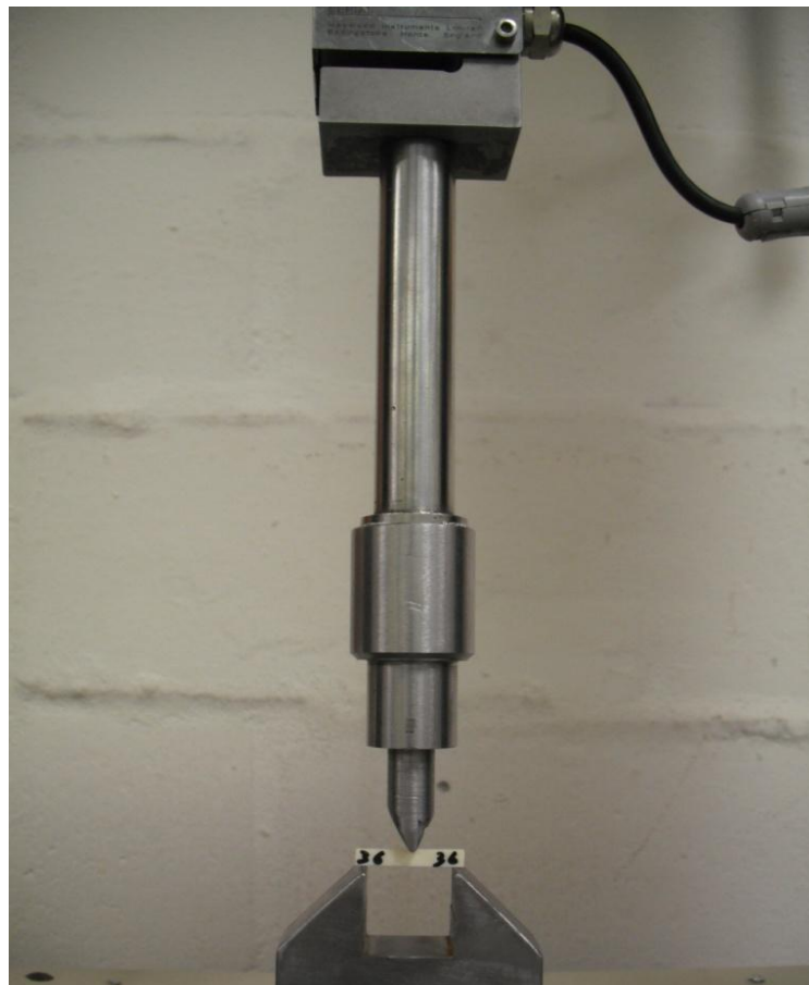
Figure 3.8: Instrumentation used for determining flexural strength
