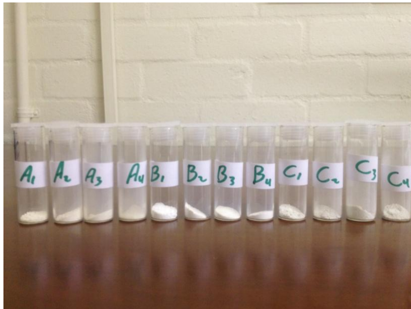
Figure 3.3: Containers with untreated and treated nano-TiO 2
