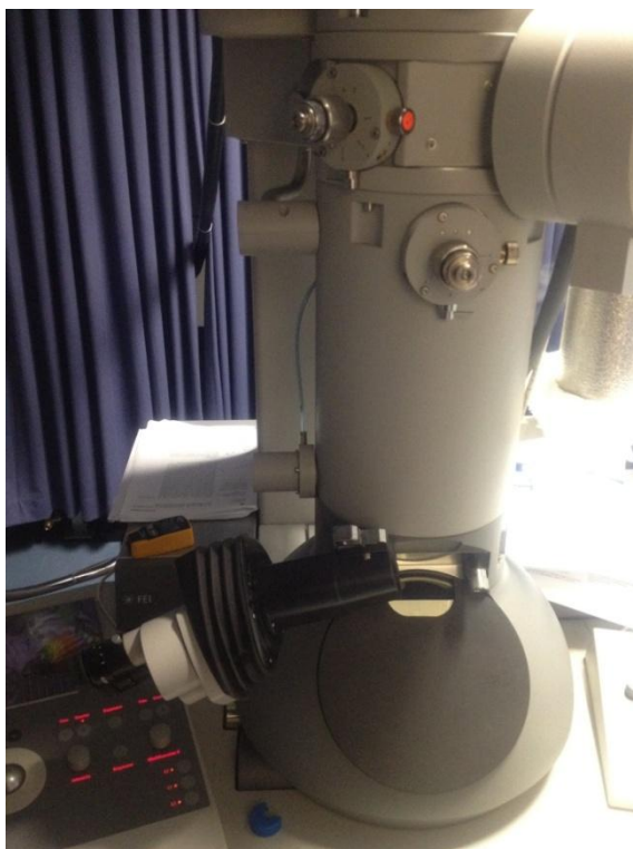
Figure 3.11: Transmission electron microscope (TEM) used in the experiment
