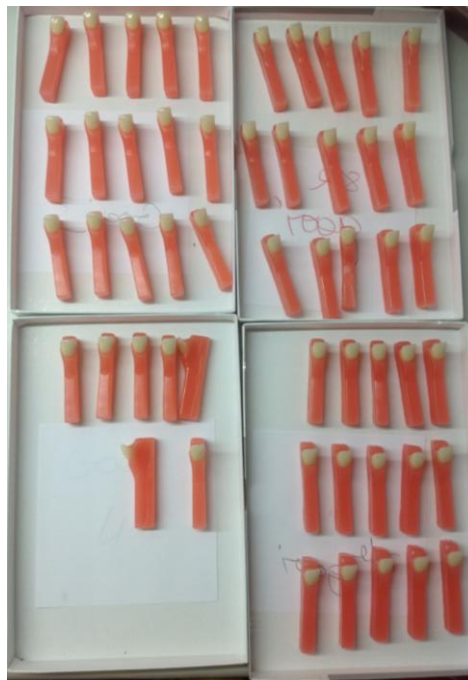
Figure 3.10: 52 exact wax replicas of the master test piece
