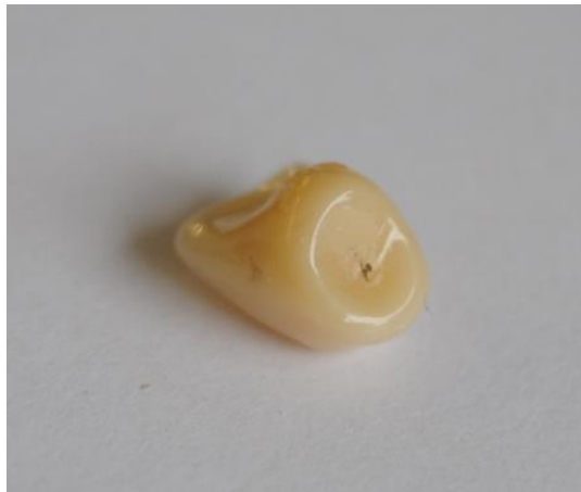
Figure 3.19: Marks in lead indicating exact drilling position
