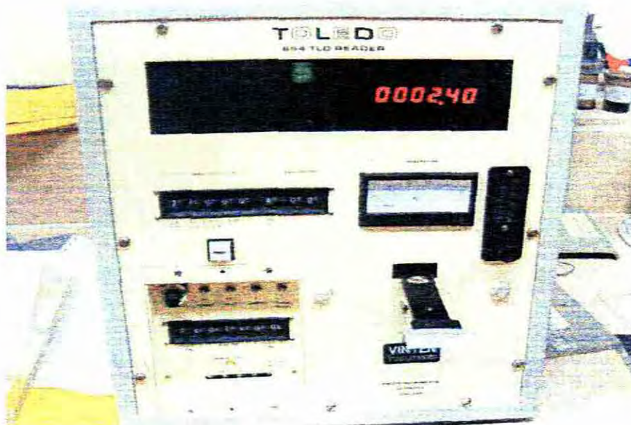
Figure 3.2. TLD reader Toledo “Model 654” Serial no. 22-5.Used for all TLD pellet readings done in this project.
