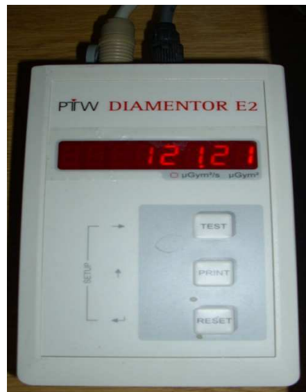
Figure 3. 2 DAP meter electrometer and display connected by a cable and operated remote from the x-ray tube at one of the study sites.
