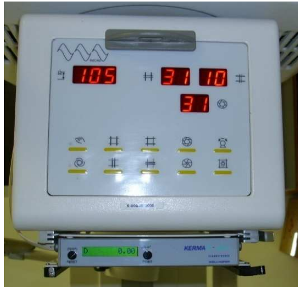
Figure 3. 1 DAP meter mounted onto light beam diaphragm of x-ray tube at one of the study sites. This DAP meter is read-out and reset in the x-ray room.
