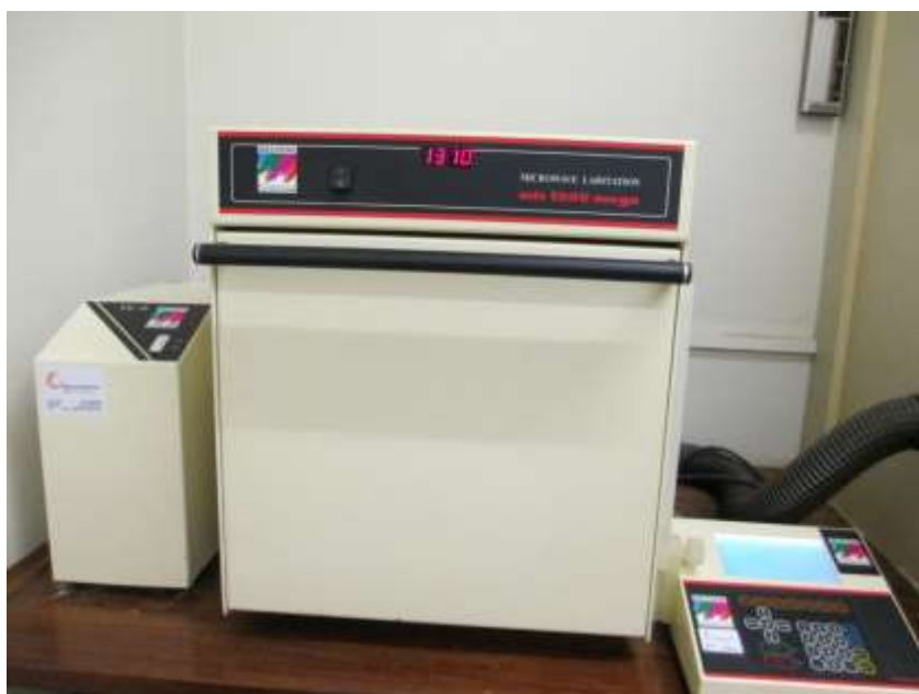
Figure 3. 3 Milestone-MLS 1200 Mega microwave oven
