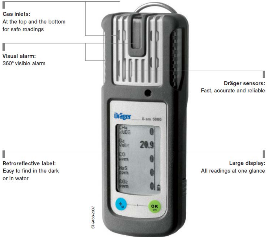
Figure 9: The Dräger X-am 5000 automatic multi gas monitor (Adapted from: Dräger Booklet, 2012)
