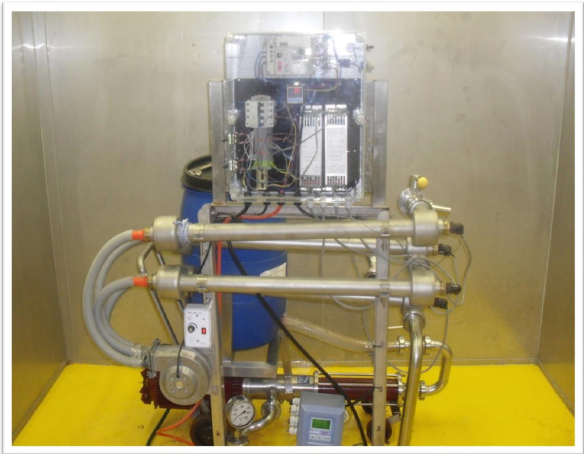
Figure 4.1: Pilot-scale UV-C reactor system used in this study
