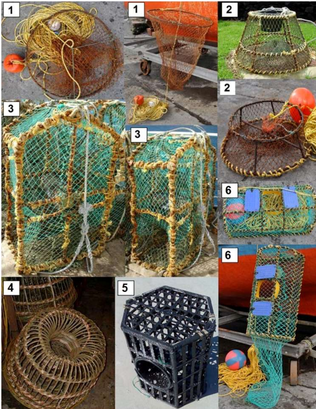
Hoop net (E.1), Bee hive or Ink well (E.2), Monster trap (E.3), Willow trap (E.4), Plastic trap or Kavel trap (E.5), Powerboat trap or pot (E.6)
