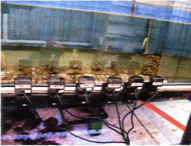
Figure 4.4: Web cams (iSonic IS-WOO1, 640x480 pixel) mounted in front of each coral fragment
