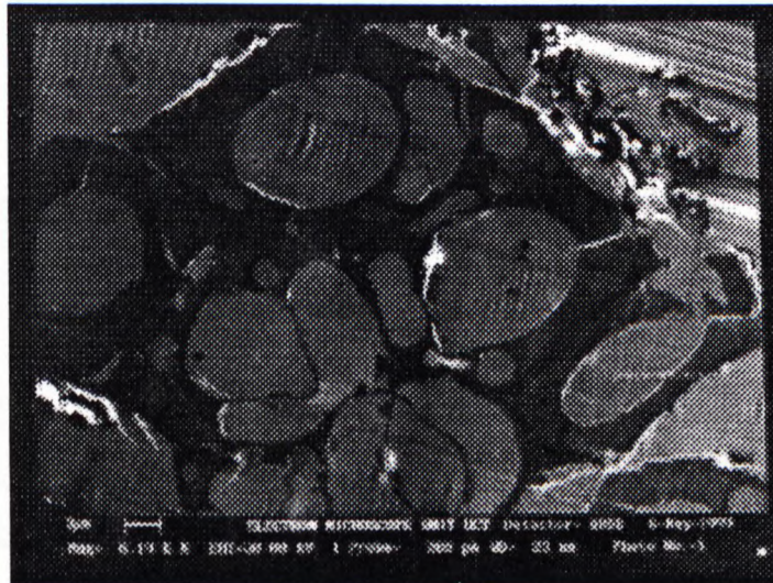
Figure 4.2 TEM of refractory wood chip showing foreign particles inside wood cells.
