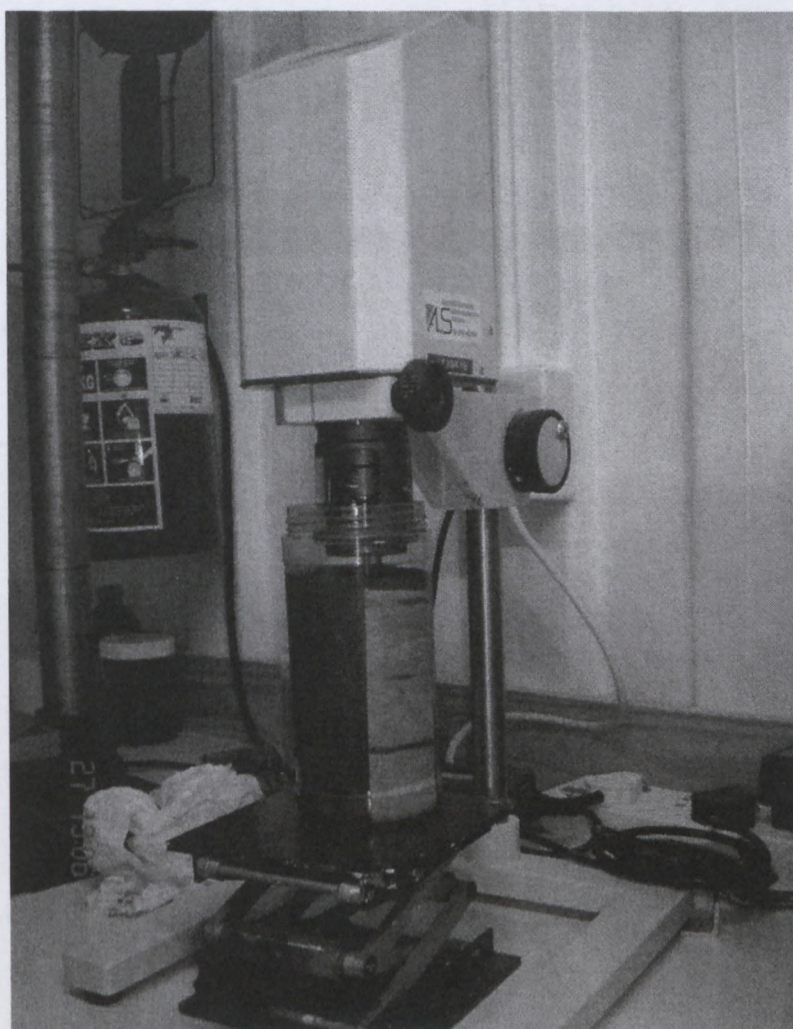
Figure 3. 4: MC 1 rheometer used for vane test
