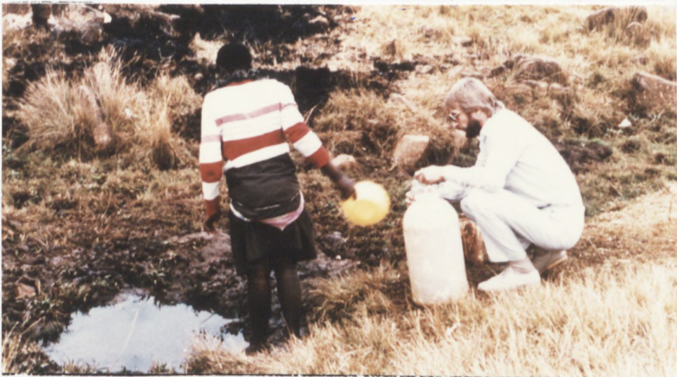
20. Mbubu - Unprotected spring. Water is collected in the pools of the small stream flowing from the spring. More than 100 faecal coliforms/100 ml .
