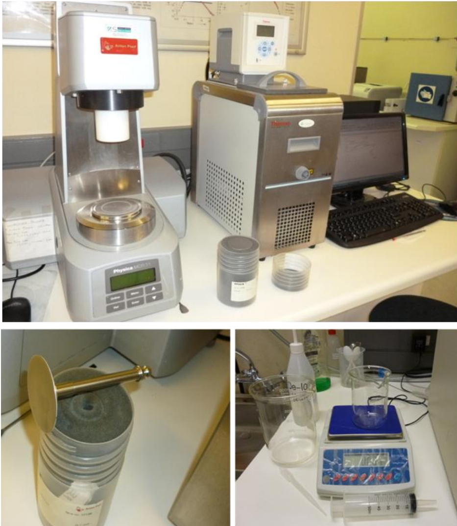
Figure 3.6: Rheometer and measuring geometry used in the experimental work
