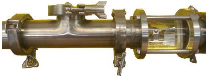
Figure 3.32: Stainless-steel flow loop glass window for in-line visual inspection
