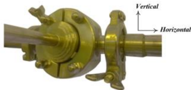
Figure 3.31: Horizontal orientation of remote seals (trapped air elimination)
