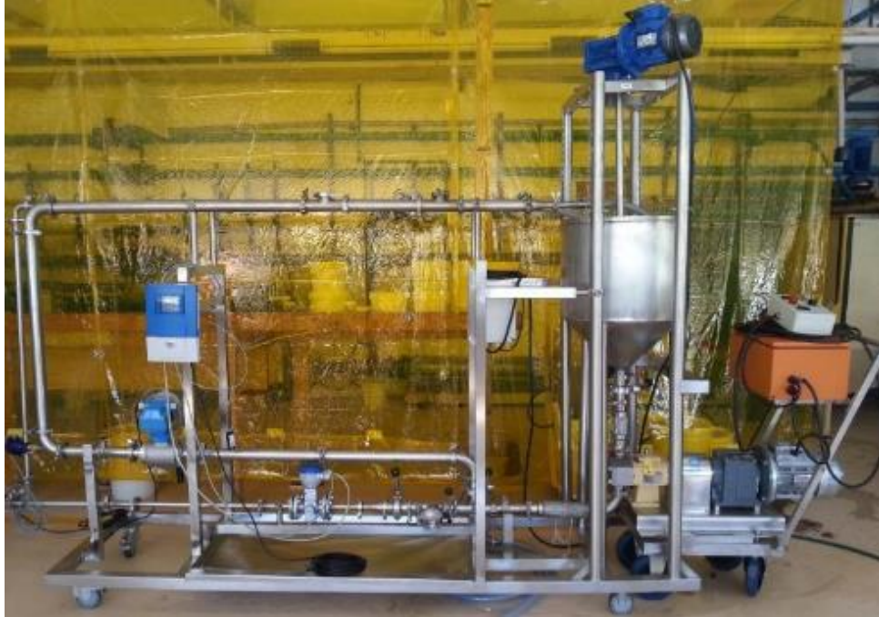
Figure 3.4: Stainless steel (316L) flow loop at the FPRC
