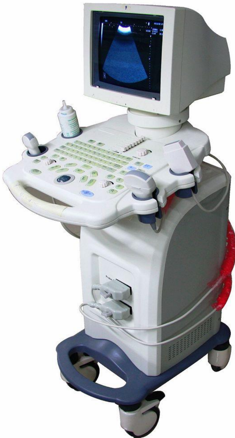
Figure 2.6 A typical medical ultrasound system (Ahmadian, 2001)
