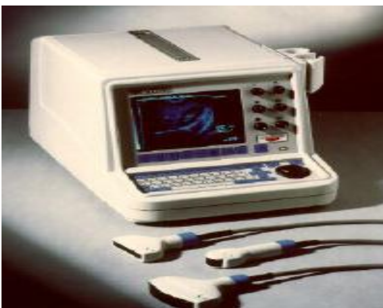
Figure 2.8 Different types of transducers (Freudenrich, 1998)
