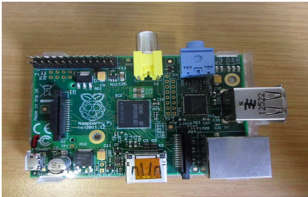
Figure 5.2: The Raspberry Pi computer used as OBC emulator in this study
