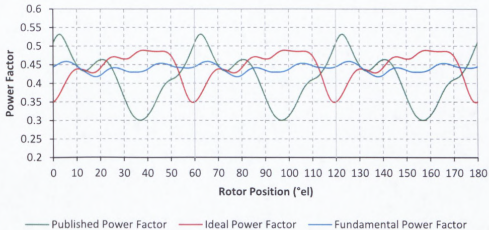
Fig. 5.3.7 Published, ideal and fundamental power factor as a function of rotor position
