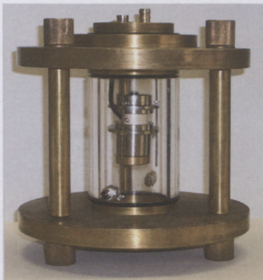
Figure 6-4: A photograph of a test rig with resonator assembled into the centre. The perspex cylinder is designed to hold silicon oil for electrical and thermal insulation
