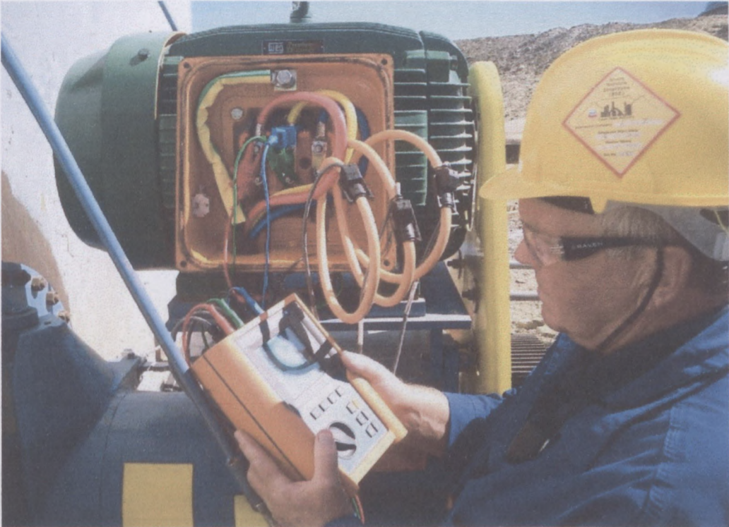
Figure 4.2 Motor test equipment connected to a motor
