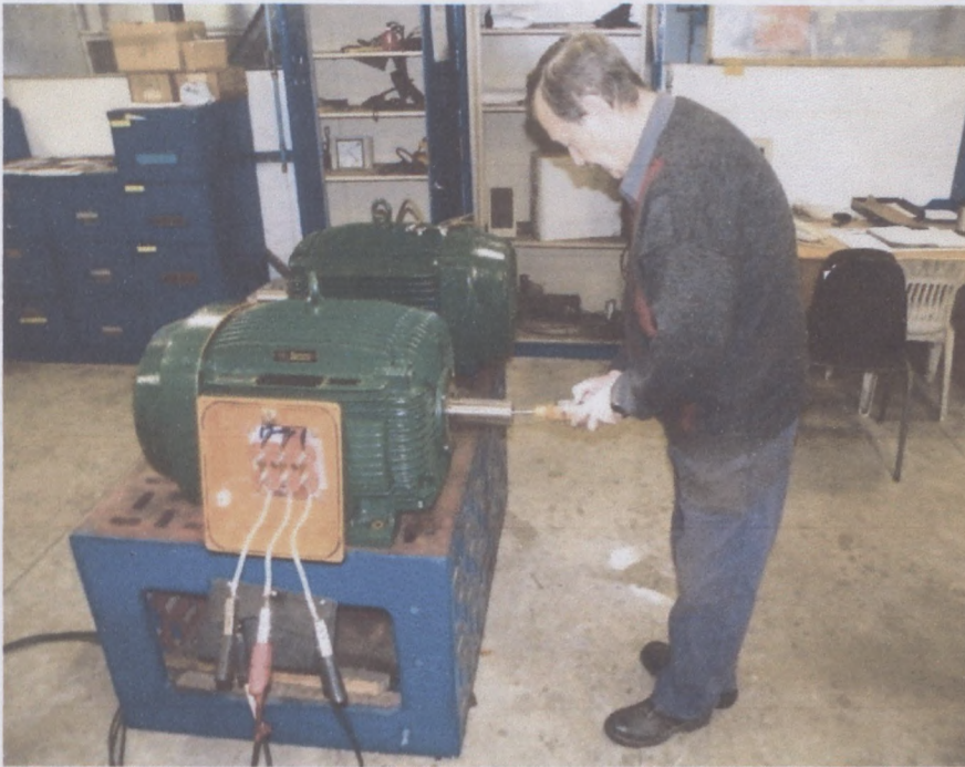
Figure 4.5 Artisan measuring motor speed with a tachometer
