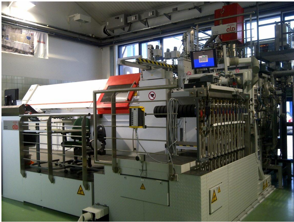
Figure 42: EB-PVD Smart coating machine.
