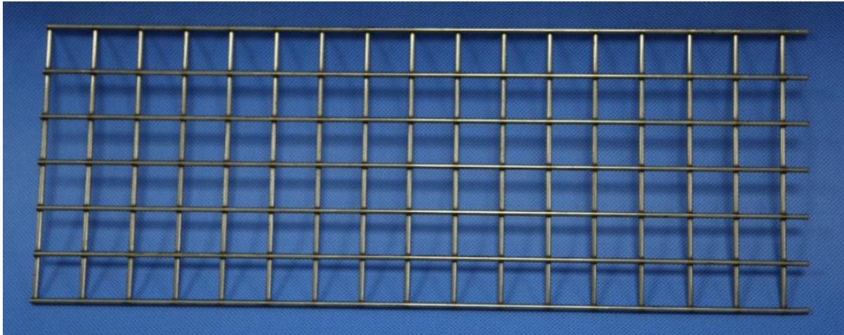
Figure 21: Wire mesh used for the distribution test (Photographed by M. Du Plessis, 2014).
