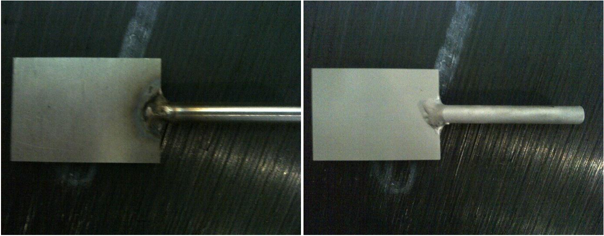
Figure 41: Flat plate sample before and after sand-blasting.
