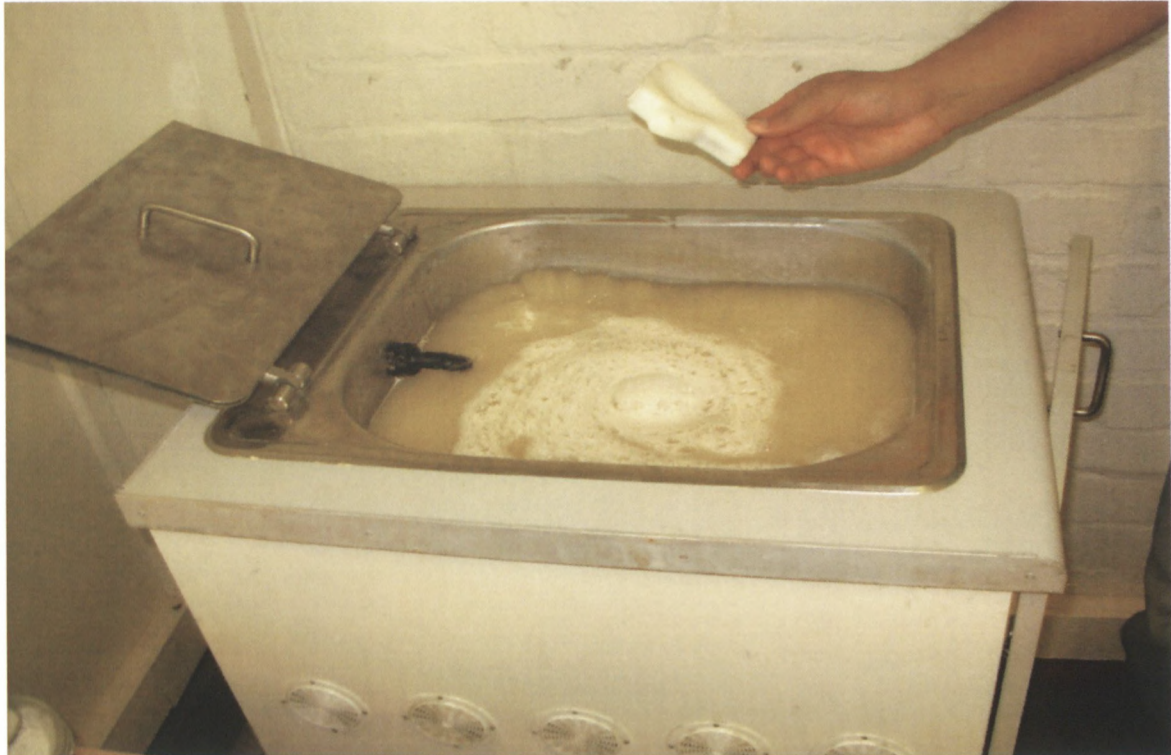
Figure 4.7: SST Station sink for washing away the support material from the palm
