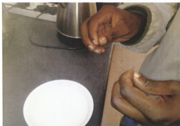
Figure 2.6: Straightening a trained Nickel-Titanium wire before immersion in hot water
