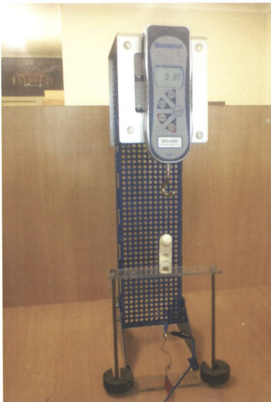
Fig 3.19a: Contraction force of each finger (3.80N)
