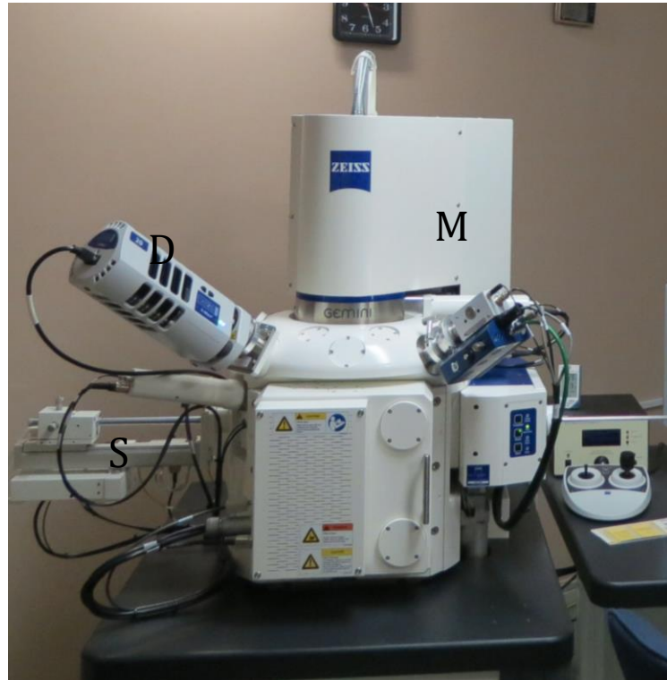
Figure 3.7: Scanning Electron Microscopy (SEM) that was used to determine the surface morphology and the Energy Dispersive analysis of X-rays is located in the Department of physics science at the University of the Western Cape, Bellville, South Africa.
