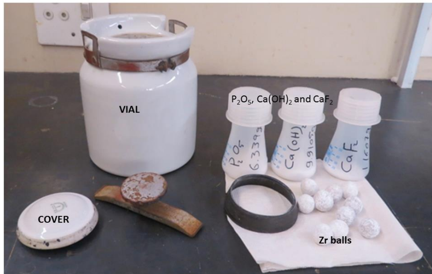
Figure 3.2: Zirconium vial and zirconium balls used for fluorapatite preparation.
