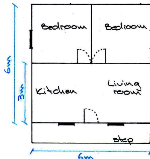
Figure A: Plan drawing of the house that was constructed indicating size and the location of door and windows (Author's construct, 2015).
