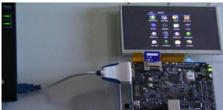
Figure 15.15: A PandaBoard with an extension board
