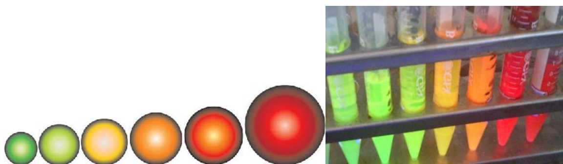
Figure 1.1 Images indicating increase in particles size of NPs as fluorescence shift from green to red region.
