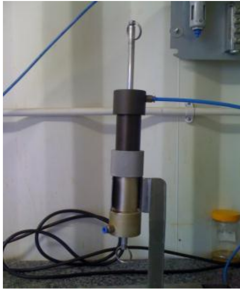
Figure 3.11: Double cylinder pumping setup
