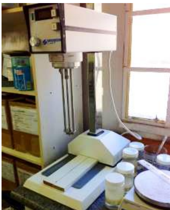
Figure 3.9: Silverson L4RT dispergator
