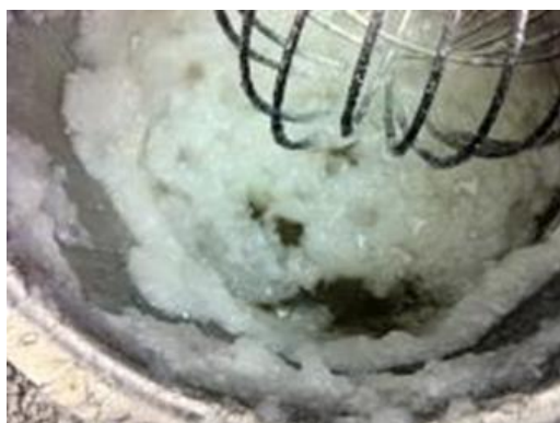
Figure 4.39: Degradation of the HCE with super cooled dispersed phase formed with the use of AM0275 POSS molecules solely
