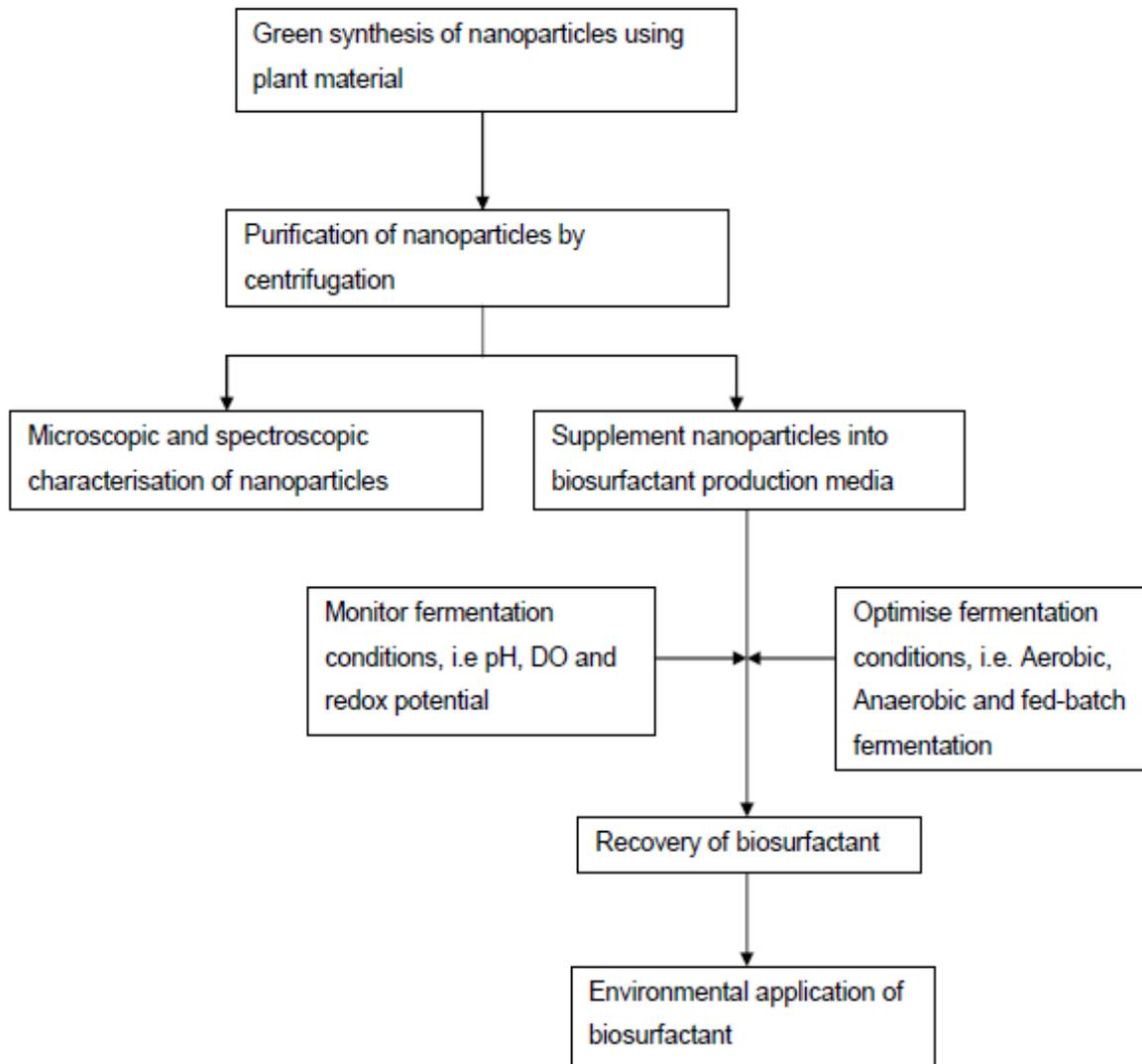
Figure 2-4: Flowchart to implement nanobiotechnology strategies to enhance biosurfactant production
