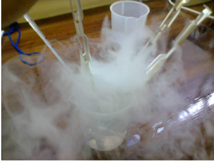
Figure 4.1: Inserting wrapped seeds contained in cryocanes in liquid nitrogen.
