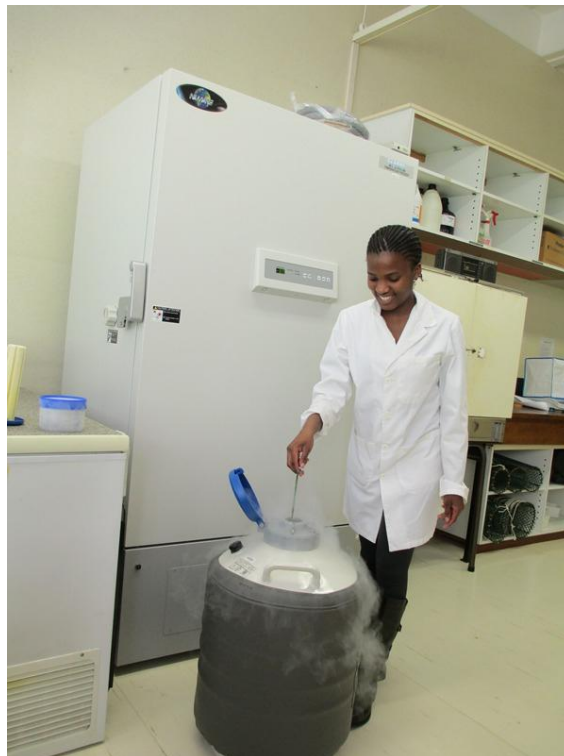
Figure 4.3: Inserting samples in the Dewar for storage
