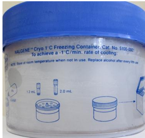
Figure 4.2: Freezing container; Mr Frosty™ freezing container used
