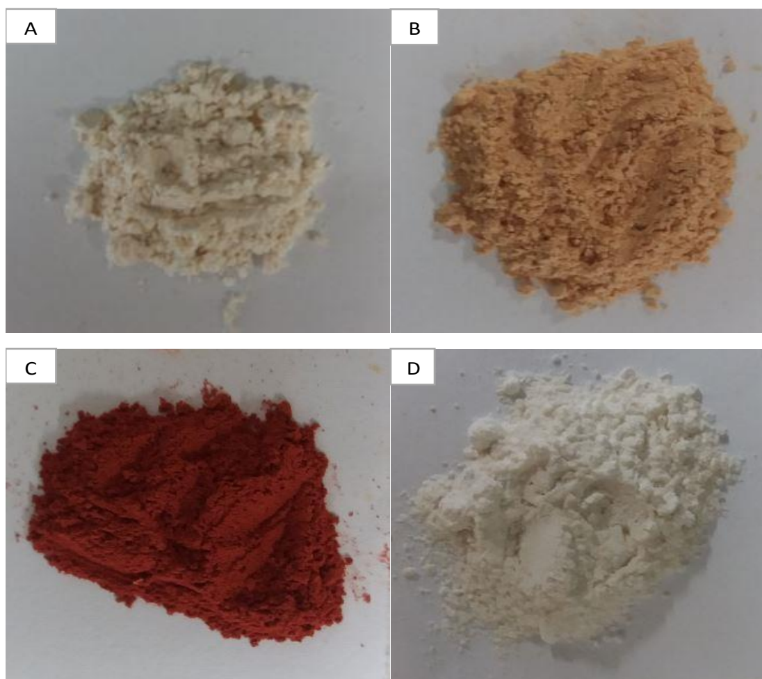
Figure 5.2: Images for the Coal fly ash alumina extracts extracted from CFA using sulphuric acid ( H_2SO_4 ), A (CFAAE1), B (CFAAE2), C (CFAAE3) and D (CFAAE4).
