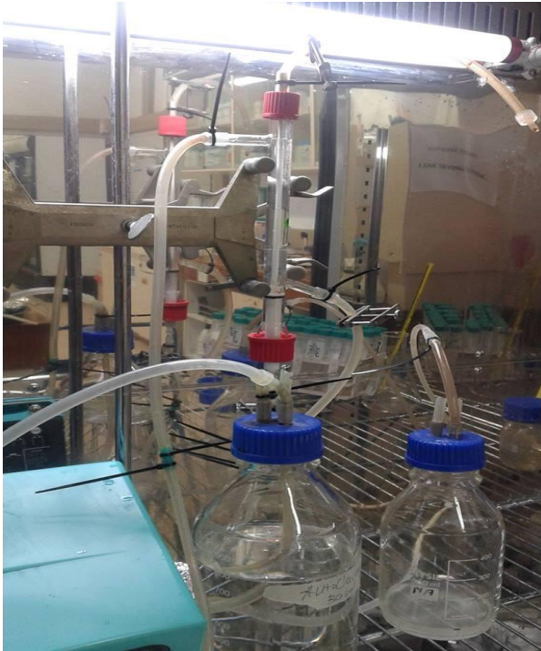
Figure C.1: Photograph of single-staged aerated membrane reactor set-up
