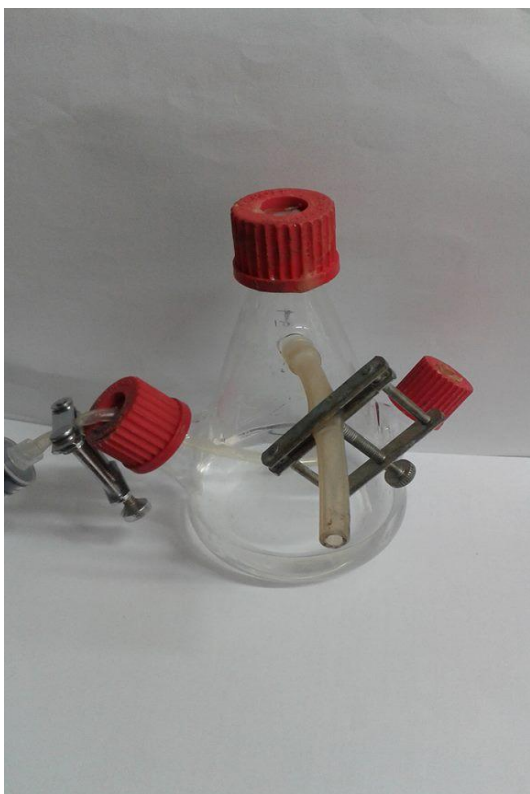
Figure A3.1 Photograph of multiport Erlenmeyer flask design used in batch experiment to avoid \text{CN}^- volatilisation
