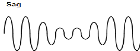
Figure 5.24: Illustration of a voltage-sag fault on a power system (Adapted from Seymour, 2011)
