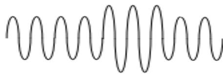
Figure 5.28: Illustration of a voltage-swell disturbance (Adapted from Seymour, 2011)
