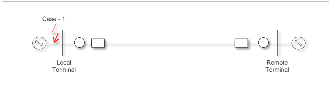
Figure 6.11: Local terminal external fault case
