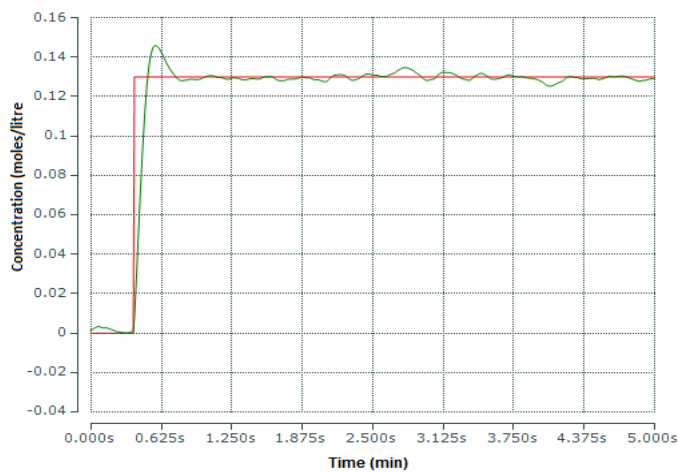
Figure 7.40: Concentration Set-point tracking under \pm 100 litres/min disturbance on u_2
