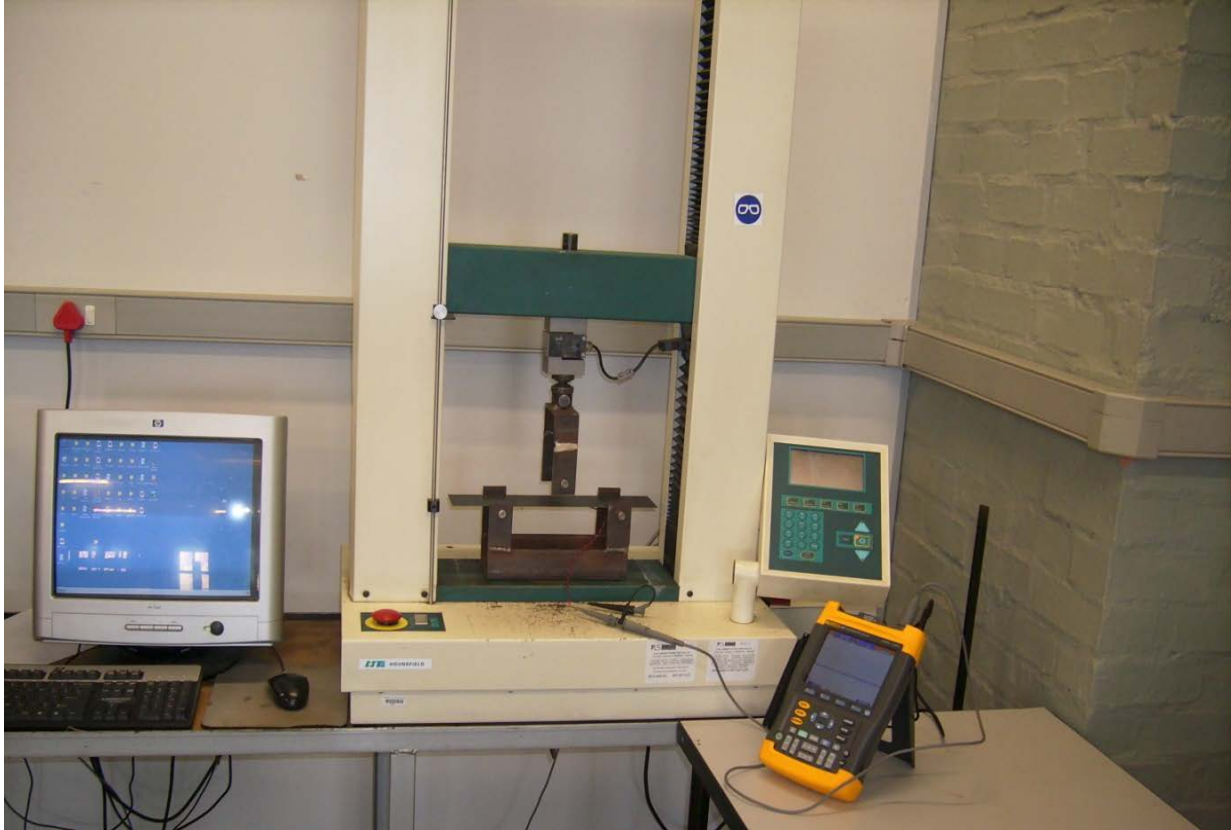
Figure 3.11: Three-point bending test with PVDF sensor attached
