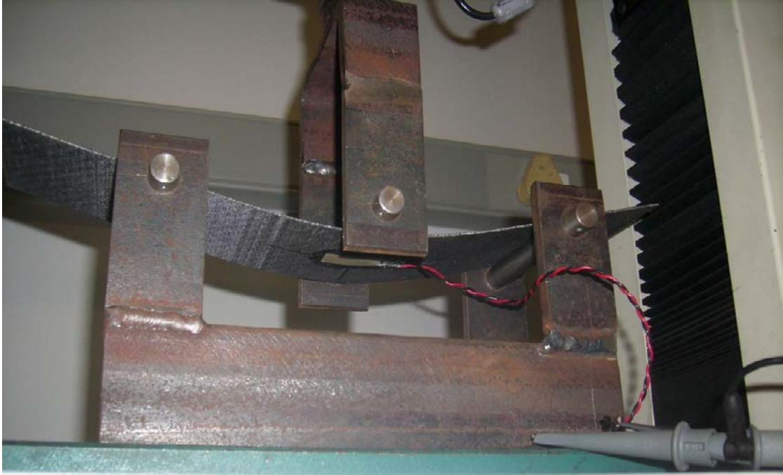
Figure 3.12: PVDF sensor attachment in a jig.
