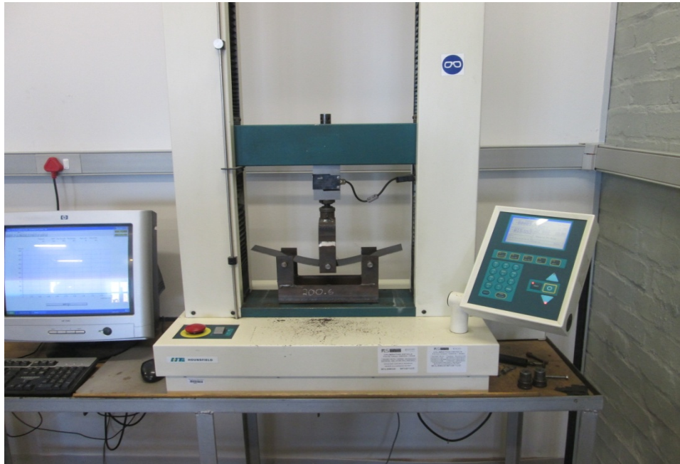
Figure 3.3: Specimen in a three-point bending test
