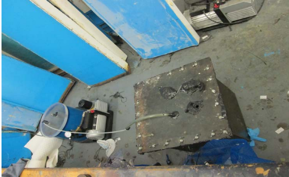
Figure 2.4: Vacuum chamber, pump and reservoir
