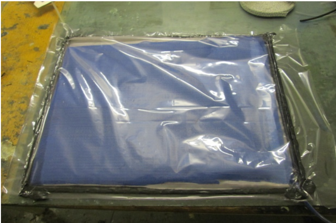
Figure 2.6: Putting the sealant tape
