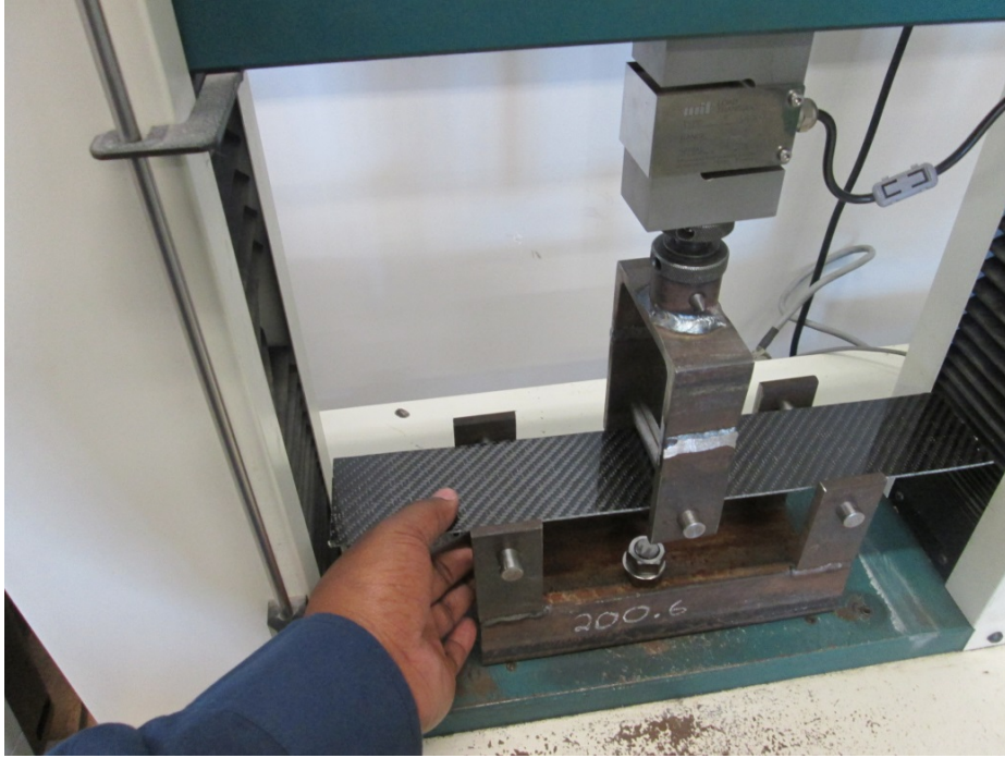
Figure 3.2: Specimen in a three-point bending jig
