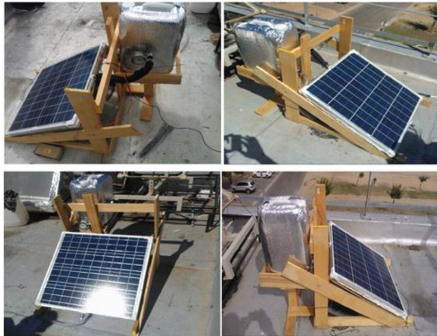
Figure 26: Constructed PV/T model for experimentation
