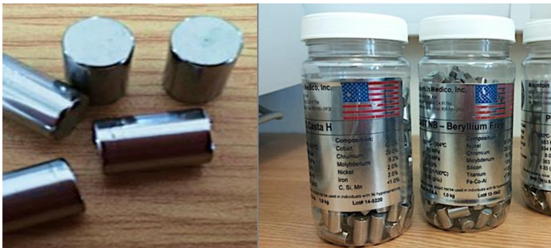
Figure 3.1: Three dental alloys PD CASTA–H, CERACAST–NB, and PD–2000, were obtained from Mountain Medico Company, Upland (California), USA. The materials were received in the cylinder–form with diameter of 7mm and 15mm length.
