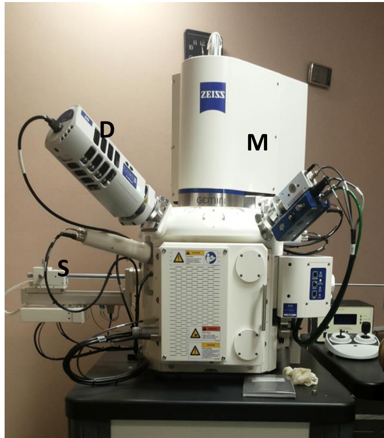
Figure 3.3: Photograph of the scanning electron microscopy SEM (Auriga Carl Zeiss, Germany) used in this study.
