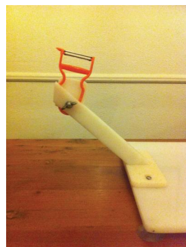
Figure 24: Initial Prototype, foundational Unit and peeler attachment (Author, 2014)
