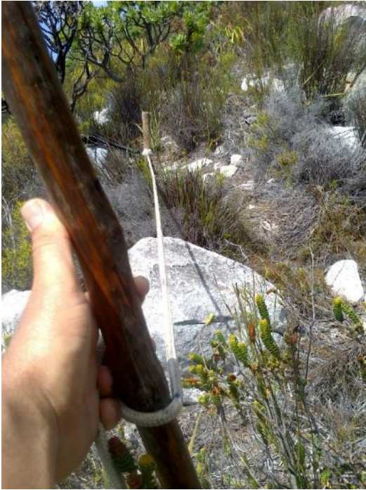
Figure 4.3: Vegetation height measurements were taken in the field at each camera point using a marked rope (1 m and 2 m), measuring stick and wooden stake (Colyn 2014).
