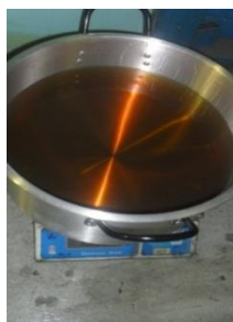
Figure 3.14: WCO to be warmed up to 55°C
