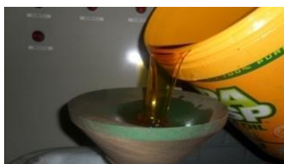
Figure 3.12: Waste cooking oil large particles filtration
