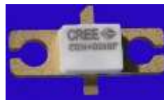
Figure 40: The Cree CGH40010F 10 W GaN HEMT power transistor
