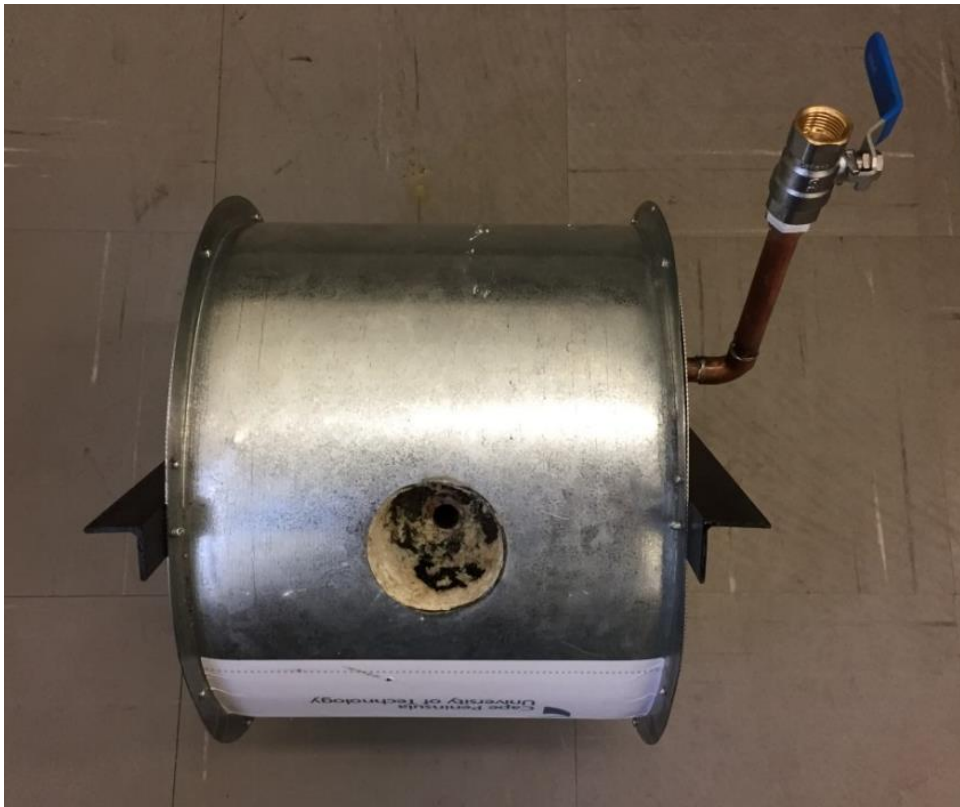
Figure 3.20: The tank for testing the heat pipe's performance
