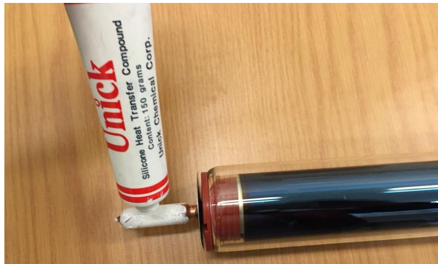
Figure 3.14: Applying silicone heat transfer compound on the bulb of the heat pipe
