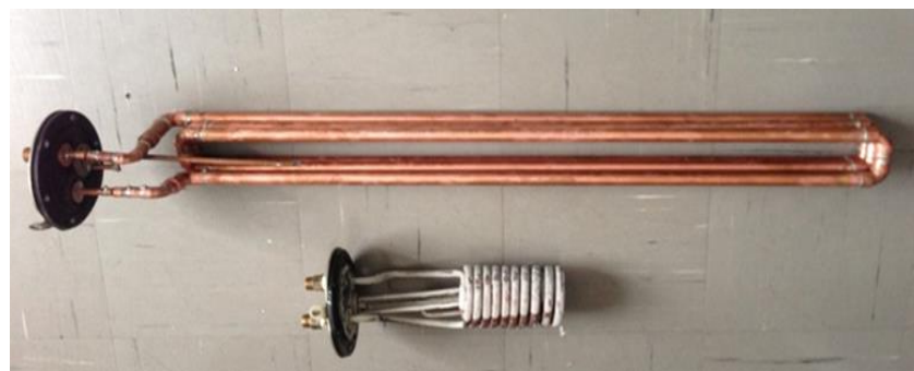
Figure 3.6: Comparison between the commercial heat exchanger with its replacement
