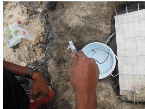
(b) Extra container close to the surface to protect the USB cable against moisture and sand particles and allow easy access for data download.
