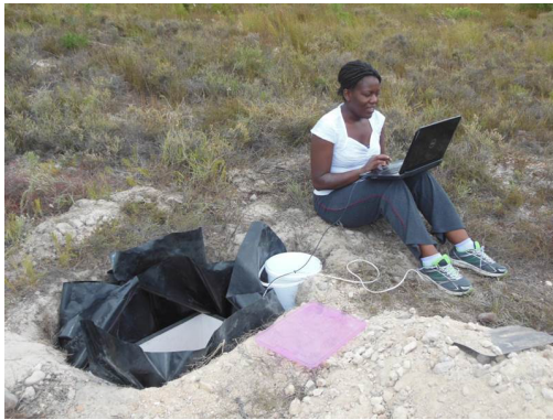
(c) Launch the HOBO data logger using a USB cable from a laptop pc.
