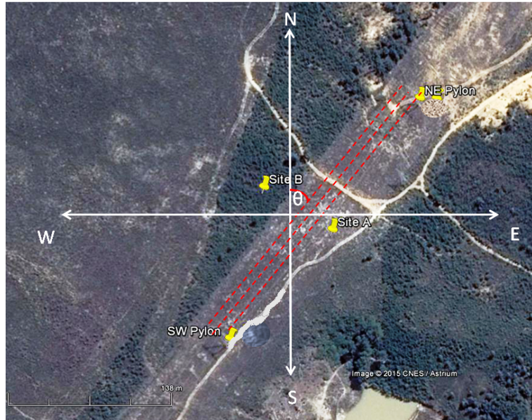
Figure 4.13: An annotated Google map image of the measurement site near Botriver which is situated \approx 30 km away from the magnetic observatory in Hermanus. The red lines are drawn along the 400 kV power lines.
