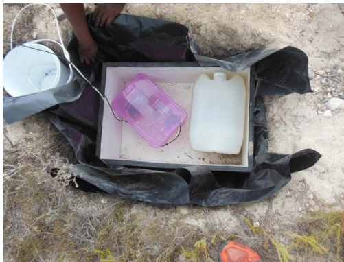
(a) Water container for temperature regulation.
