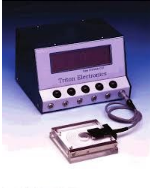
Figure 2.5: Capillary suction time device (model 319 Multi-purpose CST) adapted from (Scholz, 2005)
