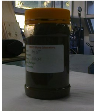
Figure 3.2: Water-tight 200 ml honey jar for sampling
