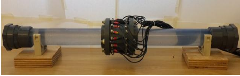
Figure 3.2 Static pipe setup fitted with two electrode rings
