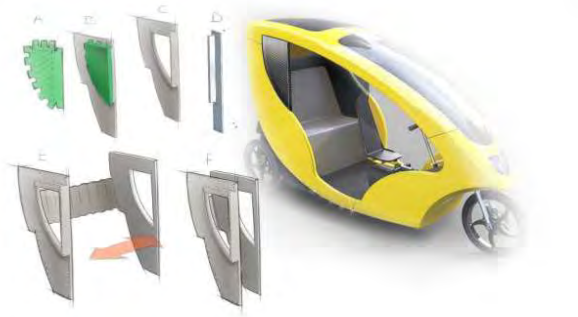
Figure 4.53: Ventilation and Low heat radiating padding (Cassim, 2015)
