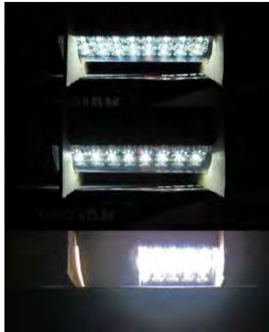
Figure 4.55: Lighting validation: Top -24, 1000 lumen SMD LED's; Middle – 8, 1000 lumen SMD LED's; Bottom 5, -1000 Lumen SMD LED's (Author, 2015)
