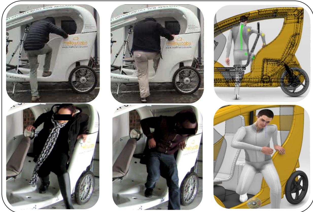
Figure 4.35: Captured movements during video analysis, simulated to drive digital manikin in CATIA (Author, 2015)
