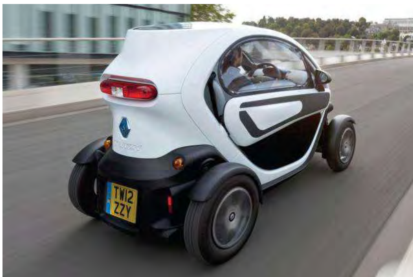
Figure 2.16: Renault Twizy fitted with door and window (Trustcar, 2014)
