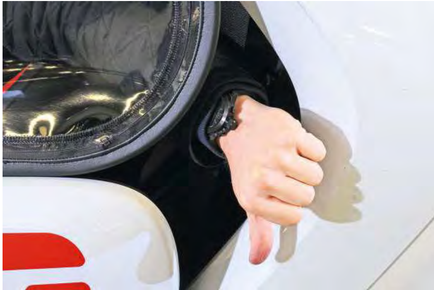
Figure 2.19: Large opening behind doors (Rix, 2013)
