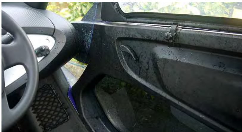
Figure 2.18: Water Ingress (Blingley, 2014)
