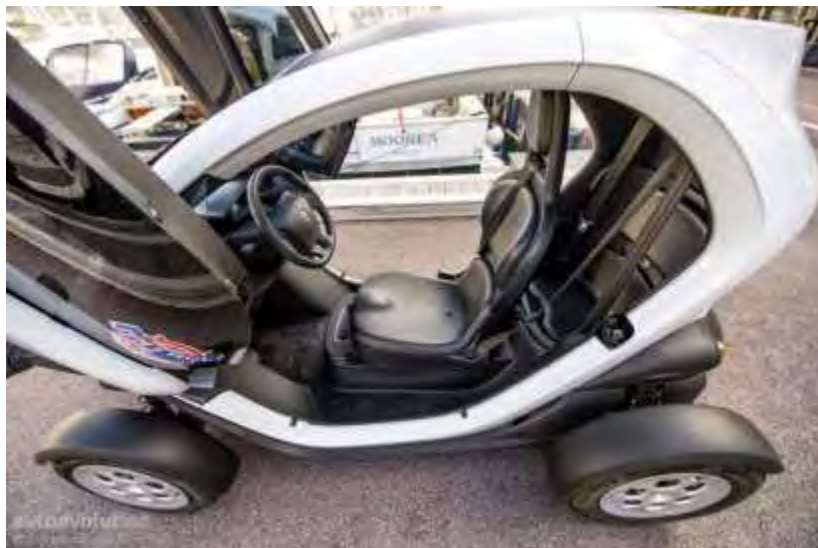
Figure 2.20: Roof rail susceptible to the Coanda-Effect (Tutu, 2012)
