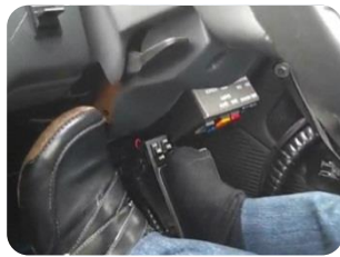
FIGURE 4.12: BUTTONS USED TO ACTIVATE EMERGENCY BRAKE
