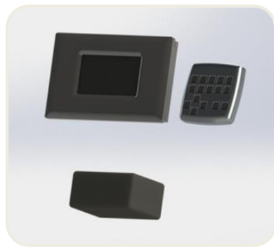
FIGURE 6.9: KEYPAD CONTROLLER AND LED SCREEN
