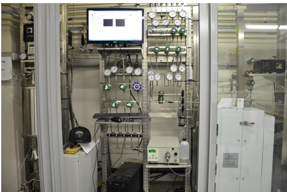
Figure 3.6 Water gas shift testing station pictorial overview
