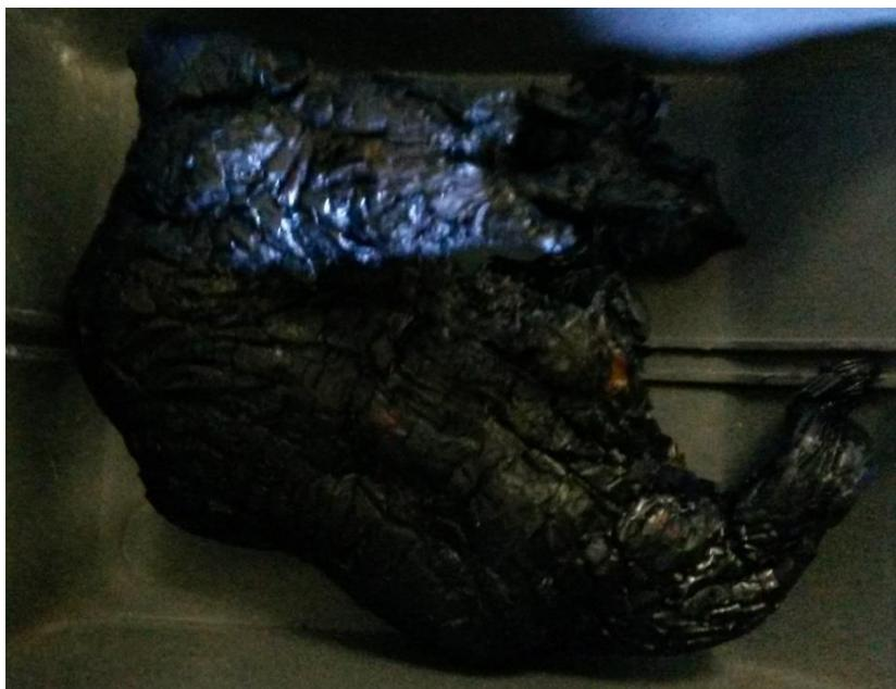
**Figure 7.12: Plastic residue after first test run. Mass of residue is 77.25 g**
