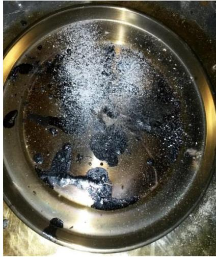
**Figure 6.5: Ash residue and char after gasification**
