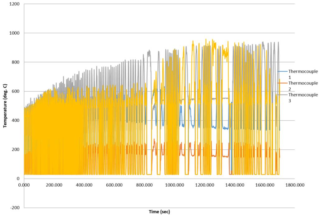
**Figure 7.36: 17 September run 3: Temperature distribution during gasification of 3 g of LDPE sample – 3 heaters on 1 heater off**
