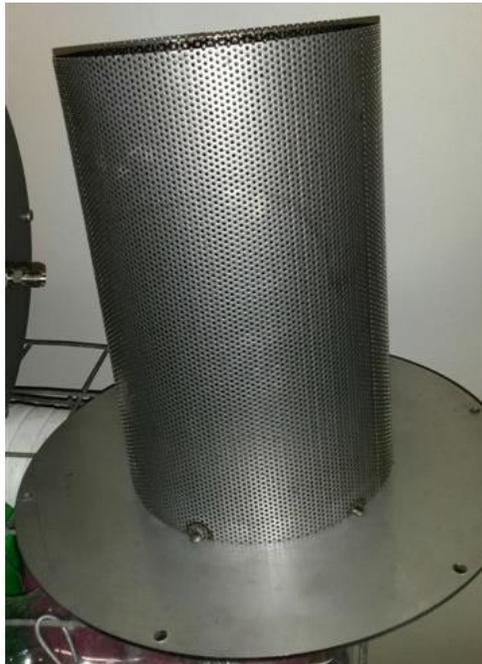
**Figure 4.12: The reactor mesh**
